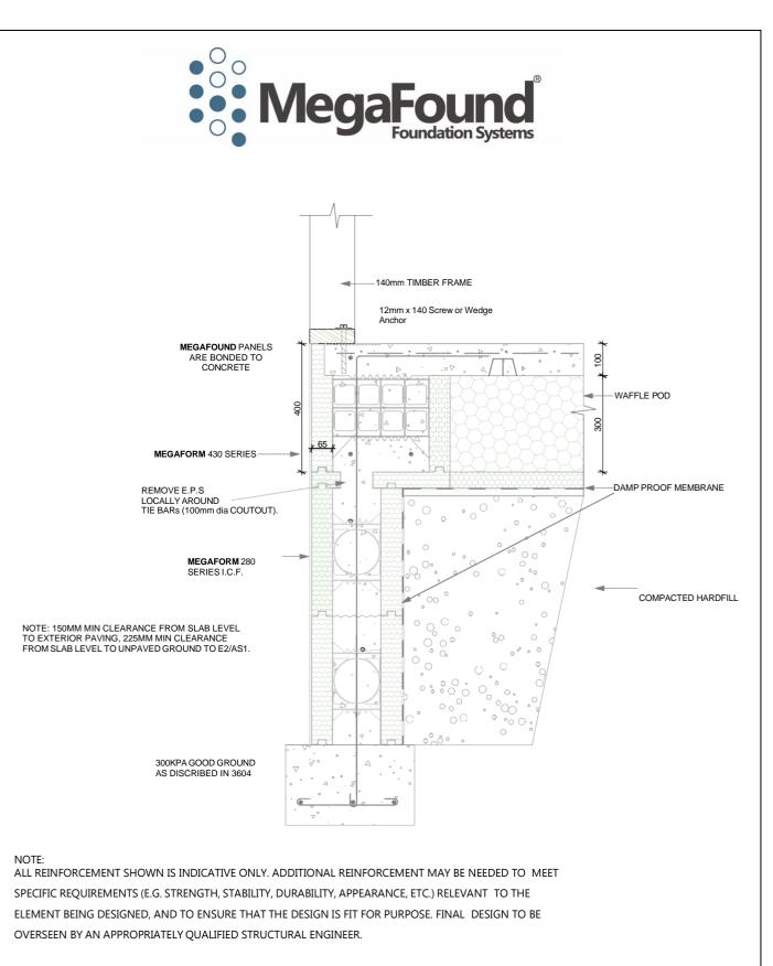
50mm EPS VH GRADE INFORMATION. COMPRESSIVE STRENGTH 165 KPA AT 10% DEFORMATION (MIN). 2% DEFORMATION GIVES 100 KPA COMPRESSIVE STRENGTH. THIS VALUE WILL ONLY EXPERIENCE 1-2mm OVERALL DEFLECTION R-VALUE 1.43.
